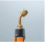
Measurement at a vent is comfortable with the bendable probe of the new testo 605i. Its thinner measurement tip is ideal for smaller measurement apertures, and the stable magnetic holder ensures even more secure attachment. The connection of the new testo 549i is angled by 45° for easier mounting.
