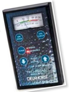
By looking at the overall ambient conditions, the contractor has a better picture of how quickly the room(s) can dry. Evaluating moisture readings taken from the moisture meter and ambient conditions taken from a thermo-hygrometer give the contractor
