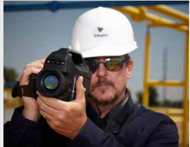
Optical gas imaging (OGI)
