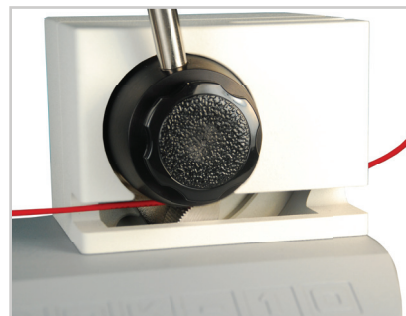
Unique knurled cam design effectively secures and pulls the loose end of the sample.
