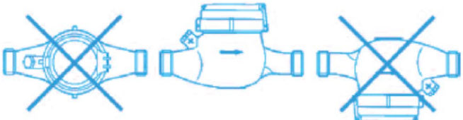
Incorrect Correct Incorrect
