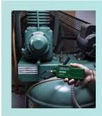
Convenient compact sized Vibration Meter measures vibration levels in industrial machinery. Misalignment, poor balancing, structural compromises, and other factors can cause unwanted vibration increases. VB450 features a wide 10Hz to 1500Hz frequency range and provides Displacement, Velocity, and Acceleration measurement.
