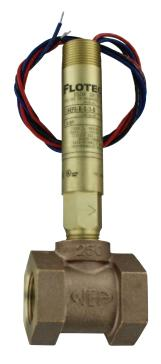
The Series V6 FLOTECT® Flow Switch is an inexpensive, explosion-proof flow switch for use on air, water or other compatible gases and liquids. Three configurations are available - 1. Factory installed in a tee. 2. With a trimmable vane for field adjustment and installation in a suitable tee. 3. Low flow models with an integral tee and adjustable valve. All are available with an optional enclosure which is UL and CSA listed, or Directive 94/9/EC (ATEX) compliant for 🕻 🕻 🔂 || 2 G Ex d ||C T6 Gb
