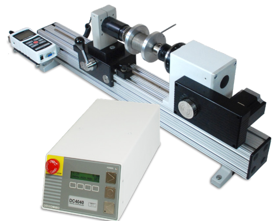
^ Model TSTMH-DC is shown in a torsion spring test, with a Series R50 torque sensor and M5i force/torque indicator
