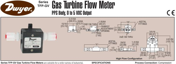
Series TFP-GV Gas Turbine Flow Meters are suitable for a wide variety of industrial, commercial, and laboratory flow applications. These meters utilize a turbine wheel and electro-optical detection to convert flow rates into a linear 0 to 5 VDC output signal for recording and data logging. Couple this unit with a Series FIV Flow Totalizer for a remote flow monitoring display. A power adapter or mating cable assembly is required for operation.
