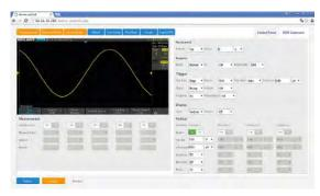
With the new embedded web server, users can control the Oscilloscopes from a simple web page. This provides remote troubleshooting and monitoring capabilities.
