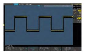
The T3DS01000 utilizes a hardware-based Pass/Fail function, performing up to 40,000 Pass/Fail decisions each second. Easily generate user defined test templates provide trace mask comparison making it suitable for long-term signal monitoring or automated production line testing.
