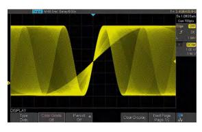
New display technology provides for fast refresh rates. The resulting intensity-graded trace is brighter for events that occur with more frequency and dims when the events occur with less frequency.
