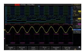
16 digital channels enables users to acquire and trigger on the waveforms then analyze the pattern, simultaneously with one instrument. Color coded logic levels clearly differentiate high and low states.
