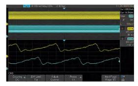
Using hardware-based Zoom technologies and max record length of up to 28 Mpts, users are able to over-sample to capture longer time periods at higher resolution and use the zoom feature to see more details within each signal.
