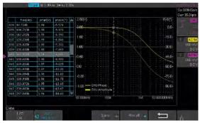
T3DS01000 can control the USB AWG module, control an independent Teledyne Test Tools T3AFG instrument, scan an object's amplitude and phase frequency response, and display the data as a Bode Plot. It can also show the result lists, and export the data to a USB disk. Not available for the T3DS01102.
