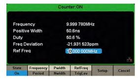
The counter functionality, accessed via the rear panel BNC, gives a DC or AC coupled counter capability from 100 mHz to 200 MHz.
