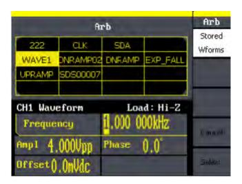
Figure 2-27 Stored Wform Display Interface
