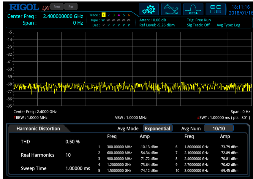
Figure 2-11 Harmonic Distortion Measurement Interface
