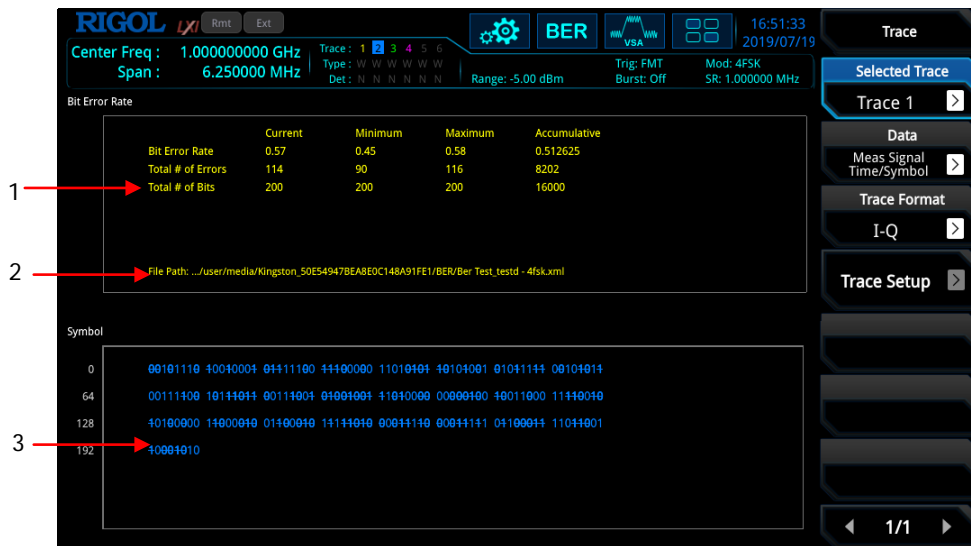
Figure 5-4 BER Measurement Results
