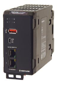
Watlow's new RMA PLUS remote access module supports Watlow's powerful EZ-ZONE® RM temperature controller family by communicating with and providing access to all EZ-ZONE RM modules in a system.
