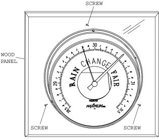
We recommend mounting the read-out on one of our pre-drilled and centered panels.
