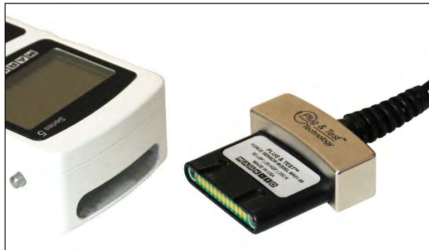
Fig. 3.1 Appropriate orientation of the Plug & Test® connector.
