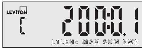
CT Amperage startup screen, no error conditions
