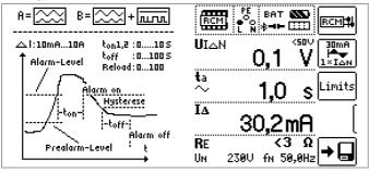
Test Sequences for Documenting Fault Simulations at type S and K PRCDs with the Optional PROFITEST PRCD Adapter
