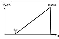
With the selector switch in the I<sub>F</sub> position, slowly rising DC current flows via N and PE. The momentary measured current value is continuously displayed. When the RCCB is
