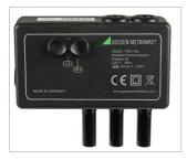
Input current: 0 ... 10 mA Input impedance: 1 k $\Omega$  ±0.5% Output voltage:
