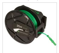
25 m measurement cable coiled onto a plastic reel. Connection to the inside end of the cable is made possible with two sockets integrated into the reel. The other end is equipped with a banana plug.
