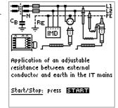
system to be monitored and ground to this end. This resistance can be changed in the manual sequence mode with the help of the softkeys, and it can be varied automatically from  $R_{\text{max}}$  to  $R_{\text{min}}$  in the automatic operating mode.
