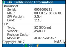
Figure 13. LinkRunner Information Screen with Connected Fiber Adapter
