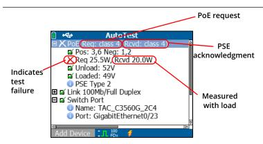
Figure 25. AutoTest results - PoE with TruePower and Measured Load
