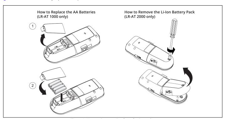
Figure 2. How to Remove/Replace the Batteries
