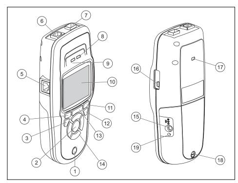
Figure 1. Physical Features of LinkRunner AT
