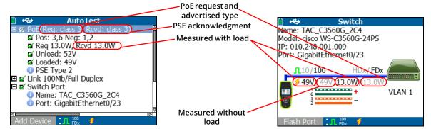
Figure 23. AutoTest results - PoE with TruePower
