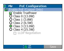
Figure 20. PoE Configuration on LR-AT model 2000
