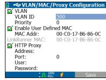
Figure 6. VLAN/MAC/Proxy Configuration Screen
