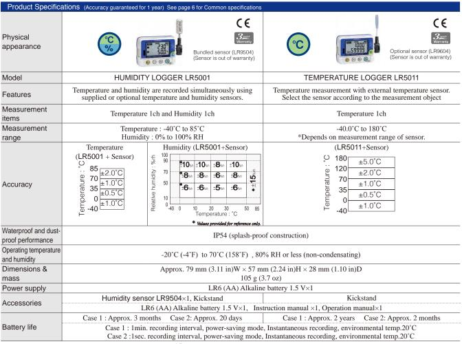
(Reference) When the recording interval is set to 10 minutes, the LR5001 Temperature and Humidity Logger can measure for about one year between battery replacements.
