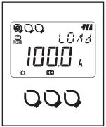
Check the connected Sensors.Sensor (P.7) and the full-scale value are displayed.
