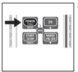
Press the button at least 1 sec. to power on the instrument. Release the button when all indications are displayed on the LCD.
