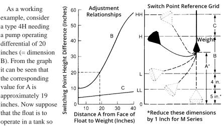
that the pump "off" position (level L) is 15 inches from the bottom of the tank. This means that the float must be hung so that the zero reference height (freehanging face of the float) is 6 inches from the bottom of the tank. The high and low alarm points HH and LL will then be, respectively, close to 41 and 11 inches from the bottom of the tank.
