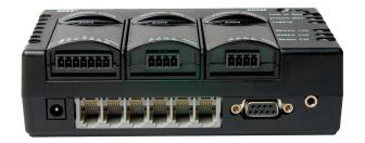
**Supported Measurements:** Temperature, Relative Humidity, Dew Point, 4-20mA, AC Current, AC Voltage, Air Velocity, Amp Hour, Carbon Dioxide, Compressed Air Flow, DC Current, DC Voltage, Differential Pressure, Gauge Pressure, Kilowatt Hours, Kilowatts, Power Factor, Pulse Input, Volatile Organic Compound, Volt-Amp Reactive, Volt-Amp Reactive Hour, Volt-Amps, Water Flow, Watt Hours, Watts, Wind
