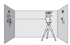
Turn the measuring tool 180° without adjusting the height.
