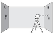
Align the height of the measuring tool (using the tripod or by placing objects underneath as required) so that the centre point of the laser beam exactly hits the previously marked point II on wall B.
