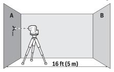
Aim the horizontal laser beam that runs parallel to the longitudinal axis of the measuring tool at the closer wall A and allow the measuring tool to level in. Mark the centre of the laser point on the wall (point I).
