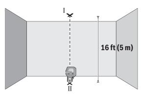
Mark the center of the top laser point on the ceiling (point I). Also mark the center of the bottom laser point on the floor (point II).
