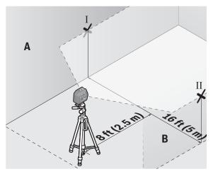
At a distance of 8 ft (2.5 m) from the measuring tool, mark the center of the laser line on both walls (point I on wall A and point II on wall B).
