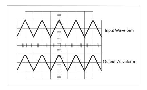
FIG 6. Amplifier overload characteristics
