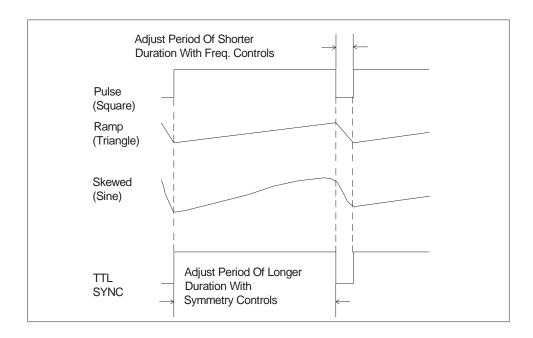
FIG 5. PULSE, RAMP, AND SKEWED SINE WAVE GENERATION
