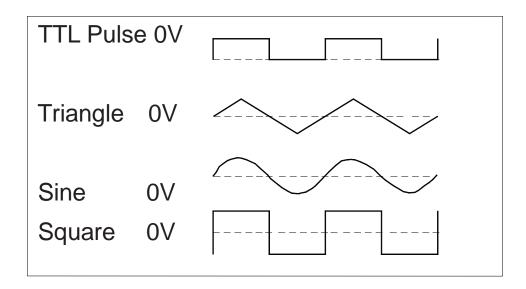
FIG. 3 OUTPUT WAVEFORMS AND PHASE RELATIONSHIPS
