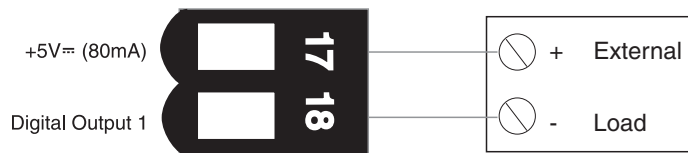
Figure 12.9c — Switched DC Example
