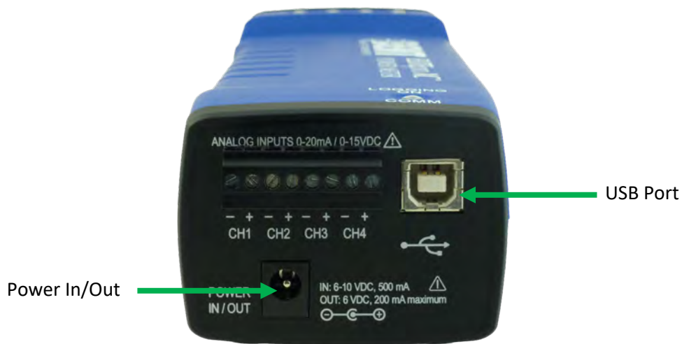
Power End Panel Connections
