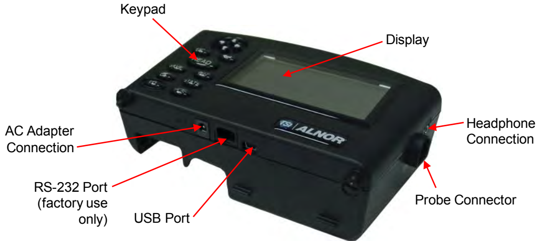
Figure 1: Features of the EBT730/EBT731 Micromanometer, Front View
