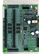
Panel 1 Set Configuration (Modbus Register 6) to Top (0)
