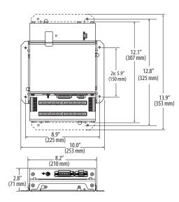
Note: The dotted lines indicate dimensions if the brackets are placed for horizontal mounting. At the factory, the brackets are placed for vertical mounting. See Installation section for more information.
