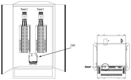
5. Connect the current sensor ribbon cables to the 50-pin connectors on the E30E. The label on the strip indicates which connector to use on the E30E (e.g. connect the strip labeled "Panel 1A" to the bottom right connector on the board). Orient the cables so that the plastic key on the E30E connector aligns with the keyhole cutout on the ribbon cable connector, as shown below.
