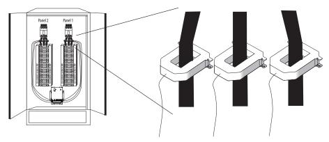
Note: The E30E measures and reports the phase angle of each voltage input and each CT (when there is active current through the primary of that CT). Use the E3x Configuration Tool to view the phase angles of active circuits to help verify that those circuits are connected to and mapped to the proper voltage phases. See the E3x Commissioning Guide (www.veris.com) for instructions on how to download and operate the tool from a PC.
