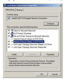
e. Select < Use the following IP Address >. Make note of the IP address that appears, then enter the static IP address (e.g. if the E30E Series is still set to its default address of 192.168.1.24, then change it to 192.168.1.100). Enter for the 255.255.255.0 subnet mask. Click OK.
