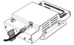
7. Once configured, disconnect the local PC. If desired (and the device is configured for operation on the network), connect the E30E directly to the network for ongoing access to the GUI even if primarily using a serial protocol to access and control the E30E.
