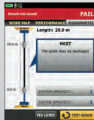
DSX-5000 uses patent-pending technology to detect connector problems.
