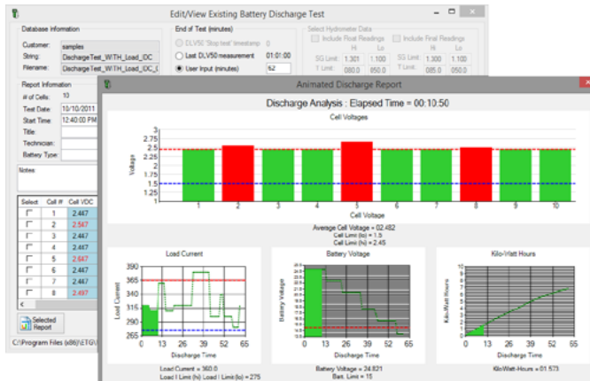
Generate Reports for Voltage, SG, and Temperature
