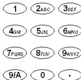
Pressing the blue key marked 9/A changes the function of the keyboard between alpha and numeric modes.
