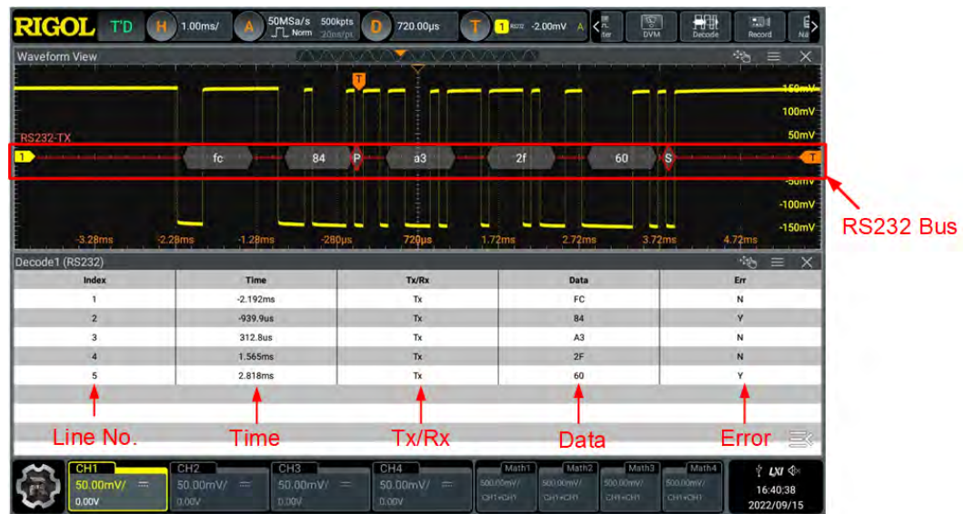
Figure 14.6 RS232 Decoding Event Table
