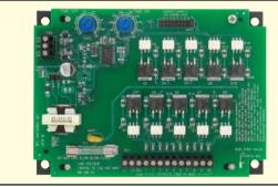
**Ideal for pneumatic conveying systems,** the Series DCT500A Low Cost Timer Controller is designed to provide continuous or on-demand cleaning for receivers and pulse jet systems. Available in either 4, 6 or 10 channels, each unit is the same size, minimizing enclosure space and reducing overall system installation cost.
