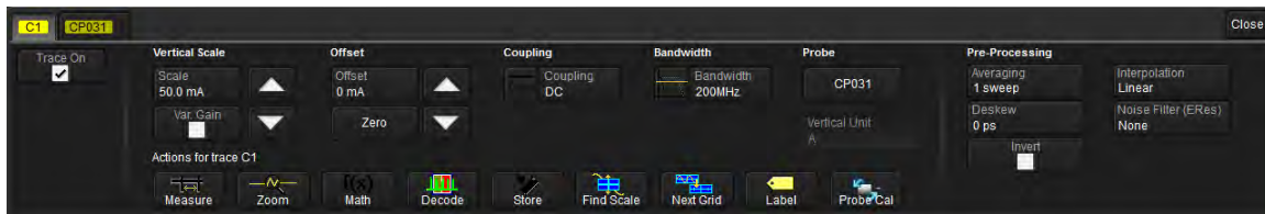
Channel setup dialog with Probe dialog behind it.
