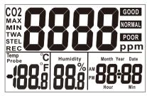
Upper LCD CO<sub>2</sub> reading Lower LCD Temp./Humidity/Real time display Carbon Dioxide reading  $C\Omega_2$ MIN/MAX Minimum/Maximun readings TWA 8 hours Time Weighted Average STEL 15 mins short-term exposure limit GOOD CO2 value is in "GOOD" range NORMAL CO2 value is in "NORMAL" range P00R CO2 value is in "POOR" range Temp Temperature Probe temperature Probe Unit of relative humidity 0C/0F Celsius/Fahrenheit of temperature
