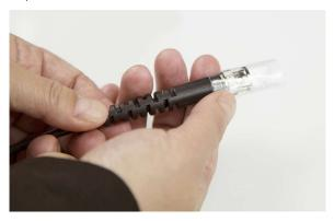
2. Connect the device to the CA10 BNC input connector.
