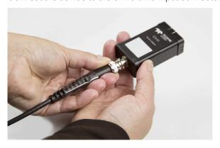
3. Slide up the sleeve so that it is flush to the body of the CA10 and completely covers the connector. Apply heat until the wrap snugly encases the connection.
