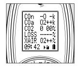
CO/CO2 displays CO (ppm), CO2, Losses calculated, Excess air %. Make any adjustments needed for proper Combustion and wait for analyzer to display change in readings. (Repeat as necessary).
