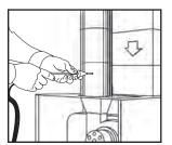
Remove the probe from the flue and allow analyzer to purge with fresh air until readings return to zero. 02 to 20.9% and CO below 20 ppm
