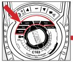
Rotate the dial to either STATUS, AUX, 02/Eff, C0/C02 or Temp setting.
