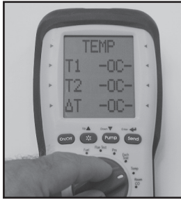
Rotate test selector to Temp
