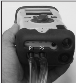
Connect true draft hose and probe into P1. Use P2 for Differential. Place probe tip in stack to measure draft. Connect static pressure hose to P1 and P2 to measure differential pressure..
