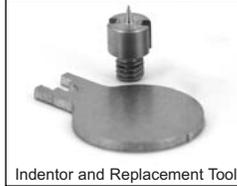
If the indenter becomes worn or damaged, a replacement indenter is included. Using the enclosed indenter replacement tool, unscrew the damaged indenter and replace. Tighten the new indenter and verify gage operation (pg. 3) before testing. A **ZERO**, **1 Pt** or **2 Pt Cal Adjust** may be required (pg. 5).
