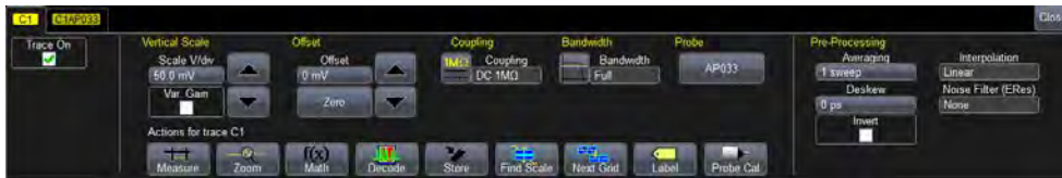
Figure 2, channel setup dialog with AP033 probe dialog behind it.
