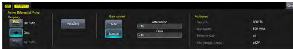
Figure 5, AP033 probe dialog with probe controls and attributes.
