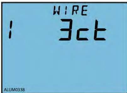
Fig.3-41 Current input wiring setting
