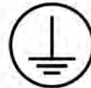
Fig 2-6 Safety Earth Symbol
