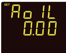
Fig 3-20 AO1 Lower Limit Setting
