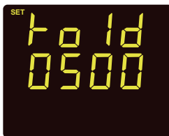
Fig 3-26 RO1 Momentary Delay Time
