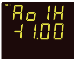
Fig 3-21 AO1 Up Limit Setting
