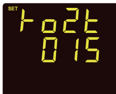
Fig 3-36 RO2 Alarm Delay Setting
