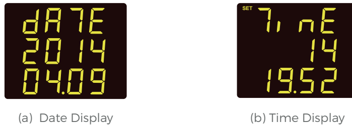
Fig 4-6 Clock Information Display
