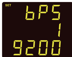
Fig 3-16 Baud Rate Setting
