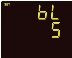
Fig 3-11 Backlight Brightness Setting
