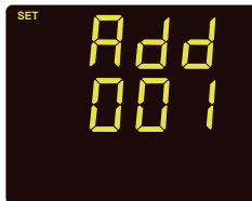
Fig 3-15 Communication Address Setup
