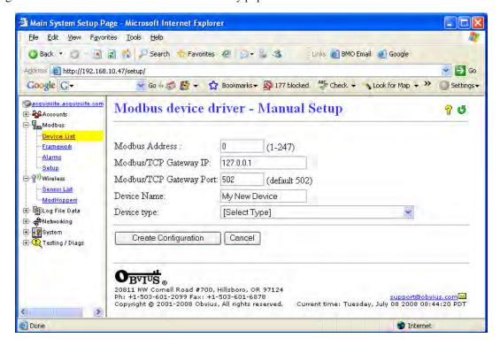
The manual setup page has several options that must be configured before the AcquiSuite will recognize the Modbus device. The options are as follows:
