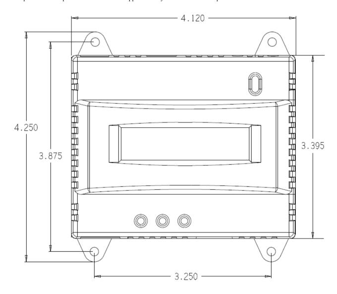
The AcquiSuite has 4 mounting holes for use with a #6 screw. The drawing above shows the relative position of the mounting holes.
