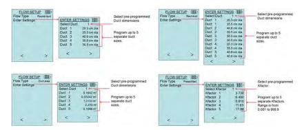
When **Flow** is set as the **Primary** measurement in the **Display Setup** menu, the dimensions or Kfactor will also be displayed:
