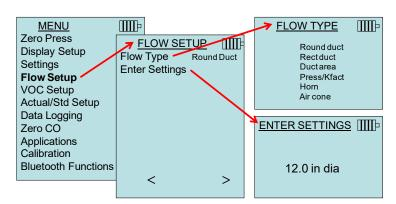
**Round duct**, **Rect duct** and **Duct area** are used to perform a duct traverse using a pitot probe or thermoanemometer probe. For more information on how to perform a duct traverse, refer to <u>Application</u> Note TSI-106.
