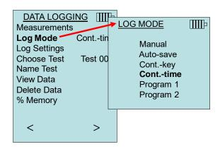
When set to Cont.-time, the log interval and test length can be adjusted.
