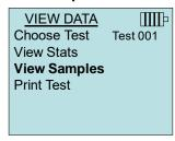
Use the ◀ and ➤ arrow keys to view samples of all the measurement parameters stored in a Test ID.
