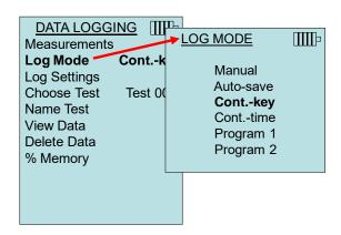
When set to Cont. key, the log interval can be adjusted.
