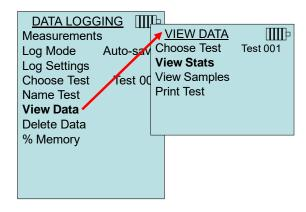
Use the ≺ and ➤ arrow keys to view statistics of all the measurement parameters stored in a Test ID.
