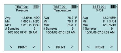
Example: TEST 001 has 9 samples, each sample consists of a pressure, temperature, and relative humidity reading. Use the < or > keys to view statistics of each measurement parameter.
