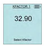
Make adjustments with the ▲ or ▼ arrow keys and press ← to accept, or enter the **Select Duct** or **Select Kfactor** menu to choose a different pre-programmed flow value or dimension.
