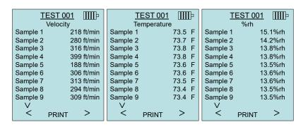
The 9565-P and 9565-X can send this data to the optional Model 8934 wireless printer or PC capable of Bluetooth communications. To use the PRINT command, Bluetooth communications must be established between the instrument and the Model 8934 wireless printer or PC set up with Bluetooth communications.
