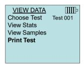
The 9565-P and 9565-X can send this data to the optional Model 8934 wireless printer or PC capable of Bluetooth communications. To use the PRINT command, Bluetooth communications must be established between the instrument and the Model 8934 wireless printer or PC set up with Bluetooth communications.
