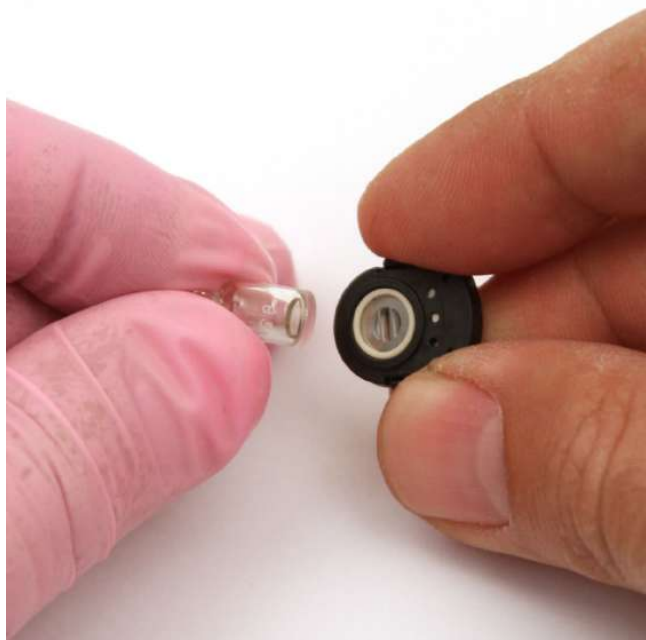
Figure 34: Reinstalling the Electrode Lamp
